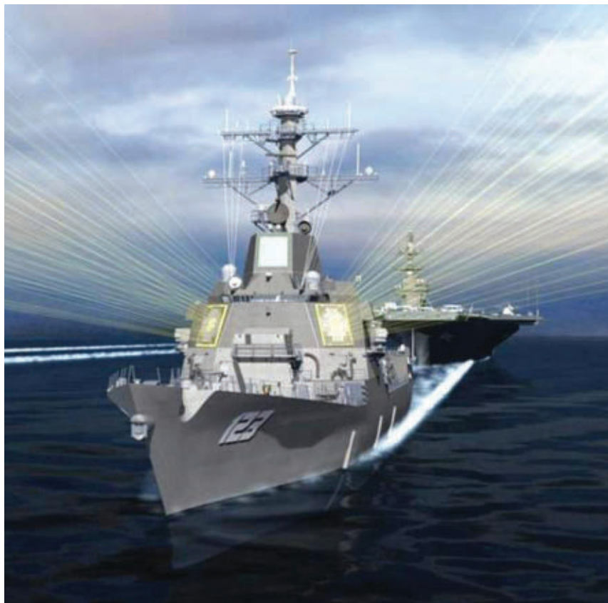
The Raytheon AN/SPY-6(V) radar will improve the Burke-class destroyer's ability to detect hostile aircraft, surface ships, and ballistic missiles.
