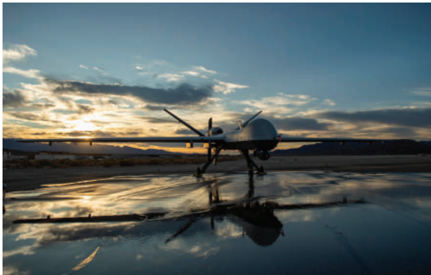
The MQ-9 Reaper is enabled by electronics that communicate with satellite systems can acquire and pass real-time imagery data to ground users around the clock and beyond line of sight. Air Force photo.
